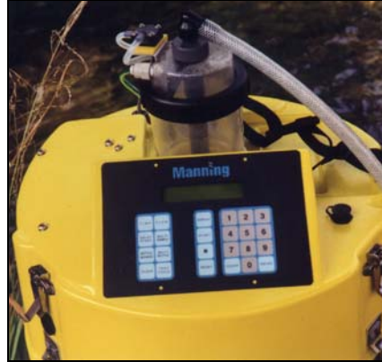
Manning VST Sampler Control Panel
